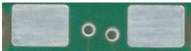
Photo: Flawless immersion tin plating layer after reflow soldering, source: Atotech
