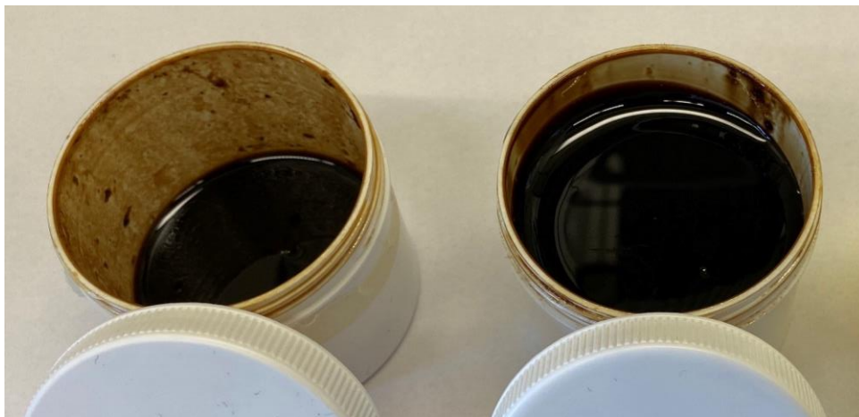
Photo: Condensate material from a condensate trap of a reflow oven at an EMS company's site – 7.7 % of weight of this brownish, semi-liquid material was identified as photoinitiator 907 by GC-MS-analysis
