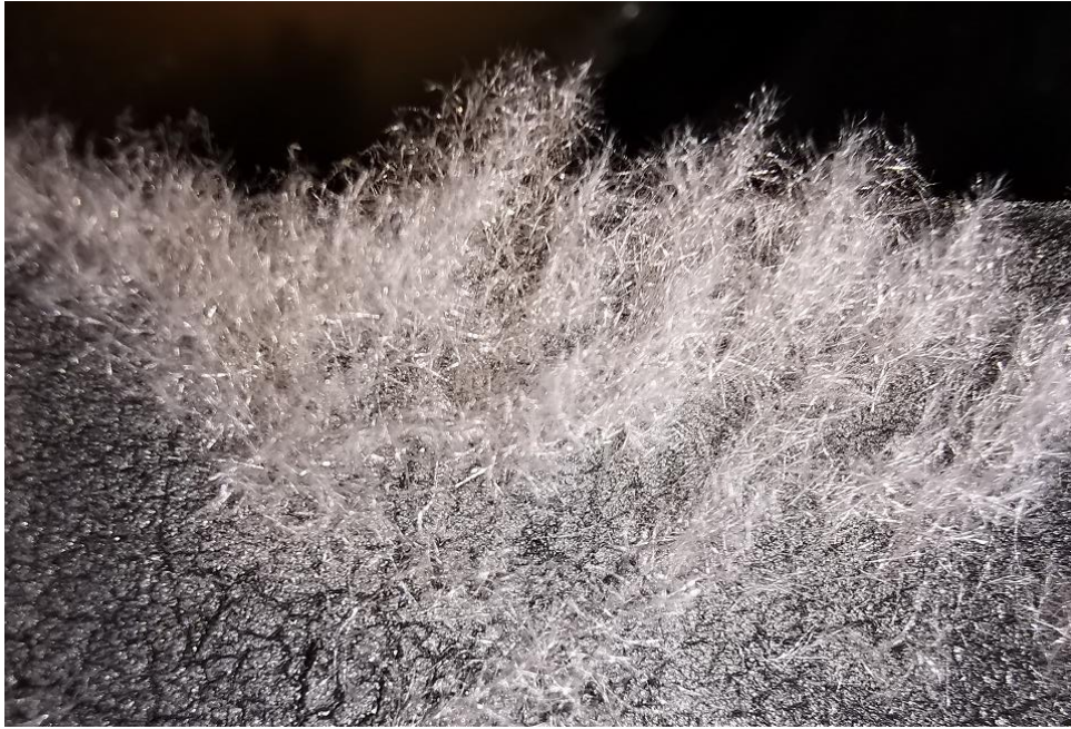
Photo: Needles consisting of photoinitiator 907 in a pre-drying oven for solder resists
