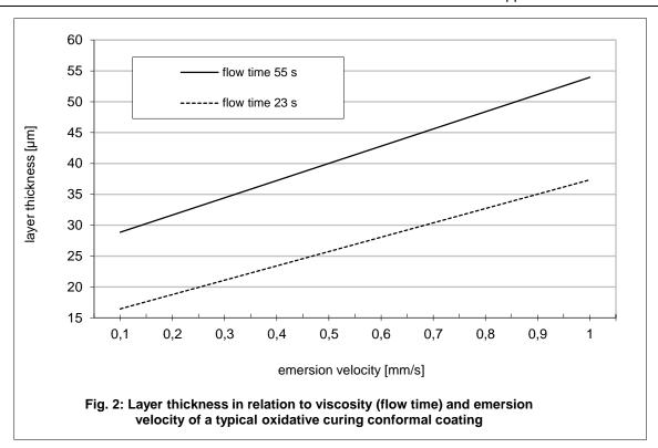
But when dip coating with a high viscosity adjustment there is a strong risk of air inclusions between the pcb and the components, besides the application of excessive coating layers (see item "Application of too high layer thicknesses/double coating).
