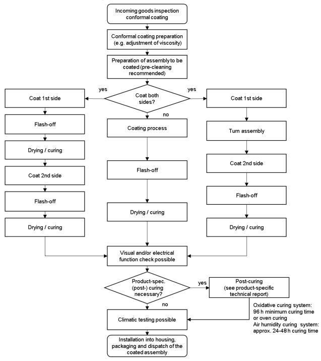
For the process steps of coating, flash-off and drying / curing one should define process-specific parameters which must be adapted to the individual unit when qualifying the process and the coating results.
