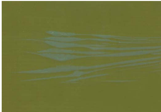
Fig. 5: Crazing in solder mask following bend stress prior to curing
