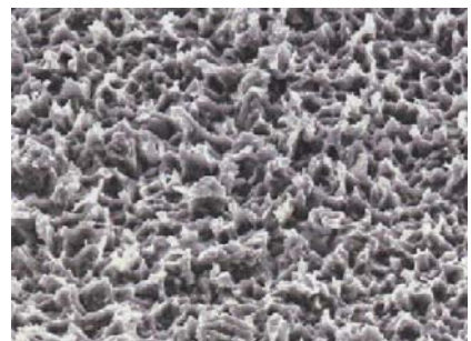
Fig. 12: Cu surface after MECetchBOND MEB
