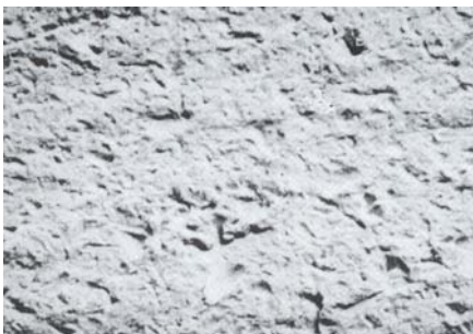
Fig. 4: Cu surface after jet pumice cleaning 2500x magnification (© IS International Supplies s.r.l., Italy)
