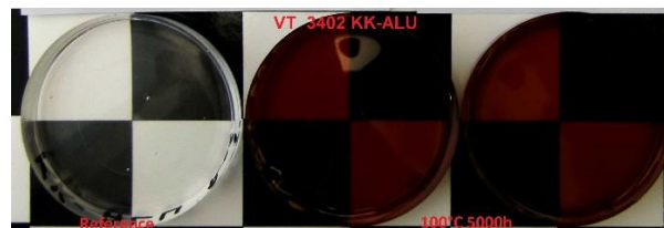
Fig. 3: Casting compound Wepuran VT 3402 KK-ALU left: Reference; right: extreme yellowing after long-term exposure to high temperature exceeding the temperature range specified
