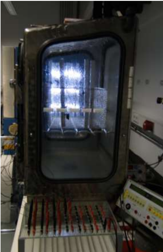
Figure 1: Climate chamber for condensation water test
