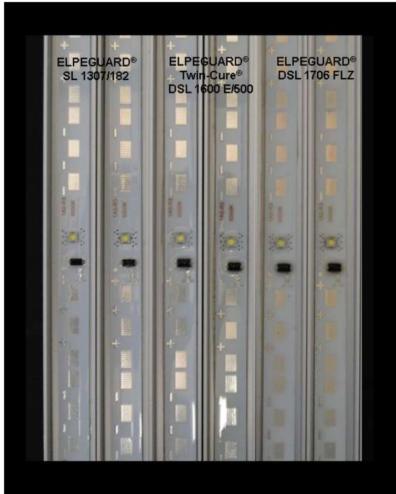
Figure 8: ELPEGUARD® conformal coatings after TCT
