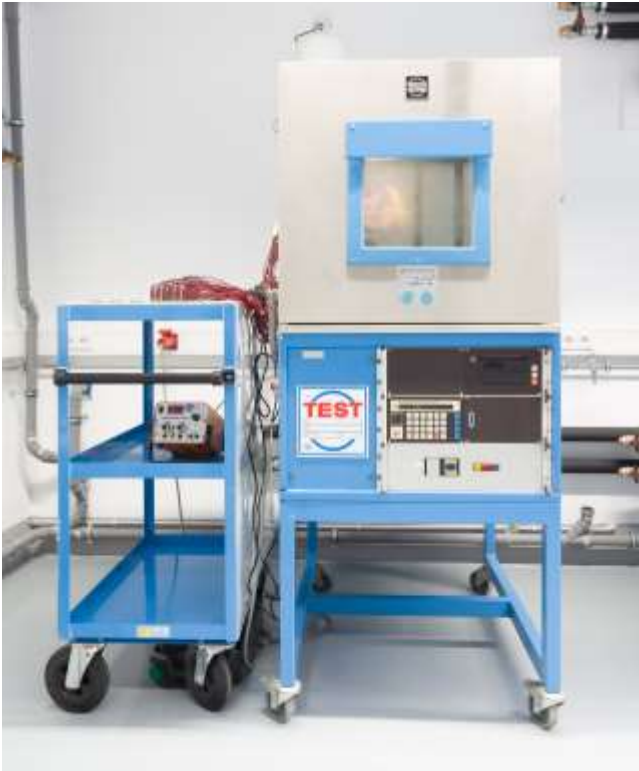
Figure 4: Climate chamber for conducting the 85/85 test
