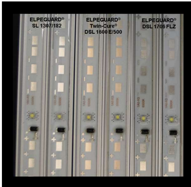
Figure 5: ELPEGUARD® conformal coatings after the 85/85 test
