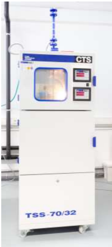
Figure 7: Climate chamber for temperature cycle tests (TCT)
