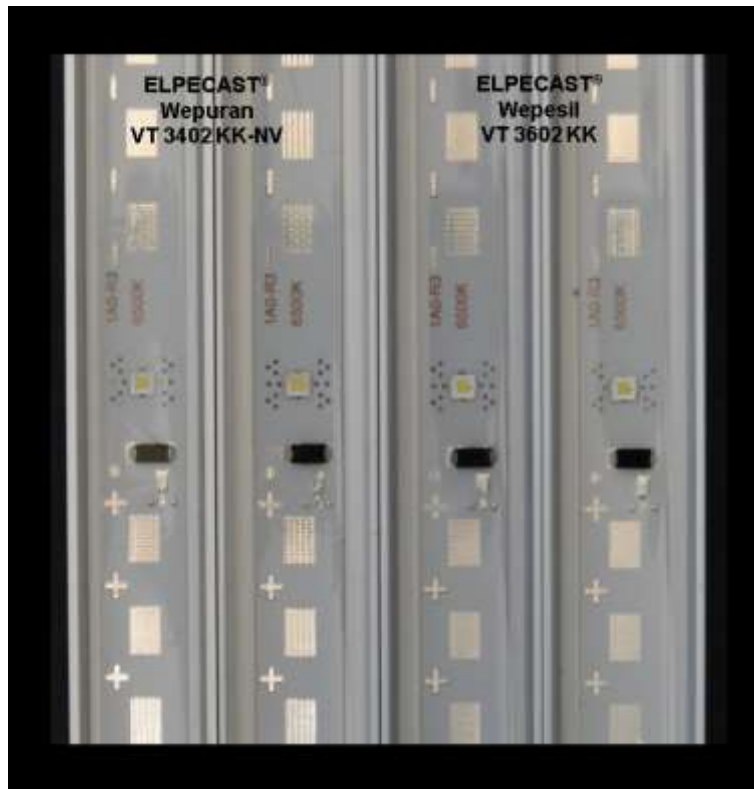
Figure 9: ELPECAST® casting compounds after TCT
