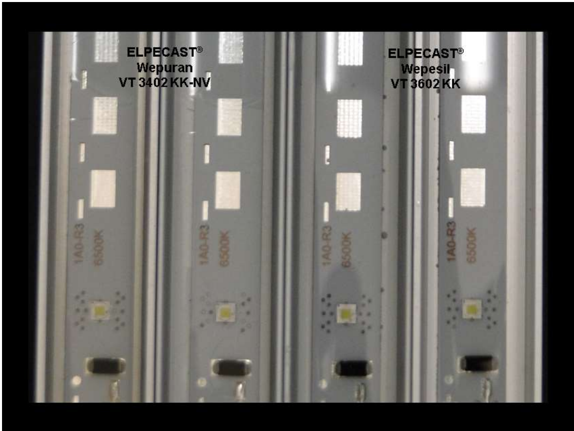
Figure 6: ELPECAST® casting compounds after the 85/85 test
