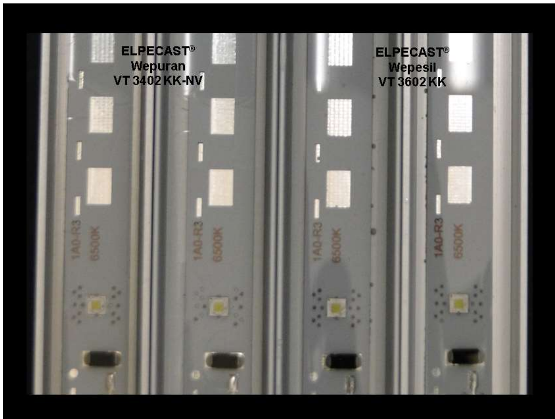
Figure 3: ELPECAST® casting compounds after the condensation water test
