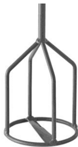
Left: Agitator with basket, right: Paddle stirrer with holes
