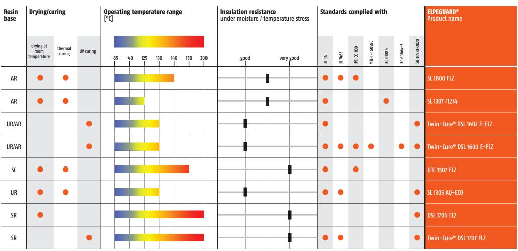
SL = conformal coating DSL = thick film lacquer ECO = ecological AQ = water-borne FLZ = fluorescent
